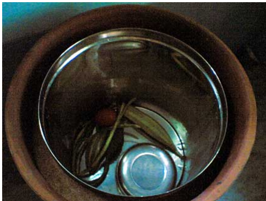
Figure 1 : Pot-in-Pot device with a stainless steel internal pot, developed at Sankalpa Research Center, Nadia.
